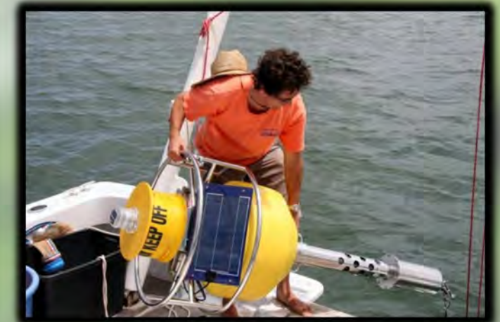
PACIOOS buoys in Hawai'i (Hilo Bay, Kiholo Bay, Honolulu) measure water temperature, salinity, chlorophyll a, turbidity and pH
